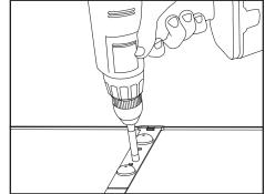
2. **Fasteners:** Use fasteners or silicone as necessary to fix LED strips into place. Refer to components list above for acceptable fasteners.
