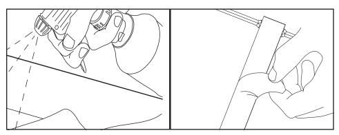
1. **Peel and stick:** Clean inside sign with rubbing alcohol and allow to dry. Using predetermined layout and LED placement from previous step, remove tape backing and stick LED strips into place. Ensure strips are firmly attached.
