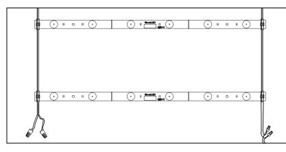
3. **Connections:** LED Strips may be connected in series or parallel, using appropriate UL/CE Listed wire connectors. Cap all unused wires. Connect power supply output to first LED strip on string. See power supply install guide for more information regarding power supply installation.
