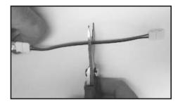
If jumper is used on terminal end to wire to power supply, jumper may be cut and stripped.
