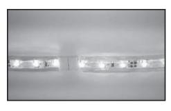
**13.** Test light material prior to final adhesion to surface to ensure integrity of all connections. Reseat connections if needed.
