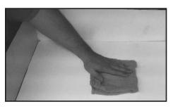
Clean mounting surface with alcohol to remove dirt and/or oil. Surface may be back of cabinet (single-sided), square tubing or extrusion (double-sided).
