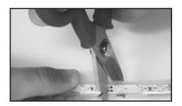
If cutting is required, cut LED strip at cut points only – designated by the line between the corresponding pair of solder/connector dots.
