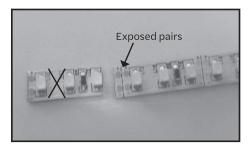
**10. For 600 LED Light Tape (PL-LT1-PW2-N-3301):**Dispose of unused section leaving four (4) connector dots exposed.
