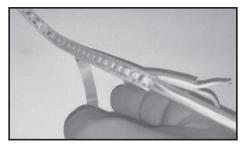
**14.** Remove release liner from VHB adhesive and adhere by pressing firmly to surface of sign.
