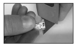
4. For encapsulated products designated "-P", additionally remove outer jacket by carefully cutting away with a razor blade to expose connector dots.
