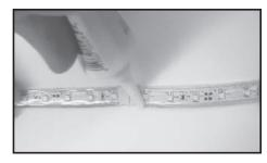
**15.** For outdoor rated (-P) material, it is critical to adequately silicone all joints and cut points to prevent water damage. It is recommended to run silicone down edge of tape to provide further adhesion.
