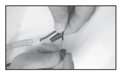
7. Once stripped, terminal end should be wired to UL Class 2 power source. Check footage chart to ensure proper loading.
