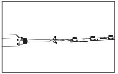
**7.** Connect to power supply: Using UL Listed electrical connectors, daisy chain product as required and connect to power supply.
