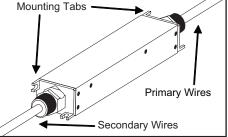
Mount Power Supply: Identify primary wires, secondary wires, and location of mounting tabs.
