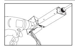
**5.** Units may be mounted in any orientation using mounting tabs.
