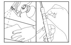
**2b.** If desired, double-stick tape can be used to mount modules. Before mounting, clean mounting surfaces inside of sign box with rubbing alcohol and allow to dry for proper tape adhesion.
