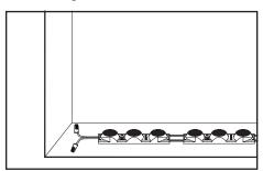
3. Fasteners: If desired, modules can be secured to sides of sign box using #8 pan head sheet metal screws or 5/32" aluminum rivets.
