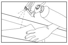
Clean surface: Clean inside of sign box with rubbing alcohol and allow to dry. Clean all mounting surfaces with alcohol for proper tape adhesion.
