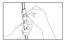
2. Peel and stick: Using provided double stick tape, mount PosterBOX Slim 2 modules to sides of sign box.
