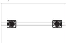
**NOTE:** For best results, space modules at two per foot. For best performance in a single-sided sign box, mount modules on returns, flush against rear wall of box. For a double-sided sign box, mount modules in center of returns.
