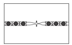
4. Connections: Modules may be connected in series or parallel. Modules should not be looped to create a closed circuit. Cap all unused, exposed wire ends.
