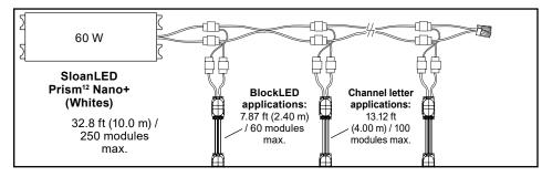
NOTE: It is recommended to connect no more than the following in series to minimize line loss:
