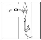
Connections: Modules may be connected in series or parallel. Tip: Discarding a module can allow longer wire lengths for connections.
