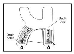
4. Back tray: Replace and seal back tray. It is important that back tray is completely sealed to prevent water entry. It is also recommended to add minimum 0.125" (3 mm) drain holes at lowest points of sign as exits for any potential water ingress. NOTE: Ensure back tray inside surface is matte white for optimum light reflection.
