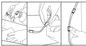
4. Peel and stick: Clean inside sign with rubbing alcohol and allow to dry. Using predetermined layout and LED placement from Step 3, remove tape backing and stick modules into place. Ensure modules are firmly attached. NOTE: If installing in a narrow channel, tape may be unnecessary. Other means of securing strip (sealant, vinyl, etc.) are also acceptable.
