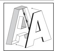
Replace sign face: Clean any debris from inside of sign and replace the sign face.
