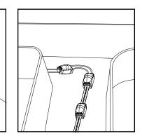
Fasteners: Use provided tape or silicone as necessary to fix modules in place.
