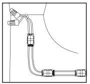
Cap all unused wires: Using appropriate UL Listed wire connectors (refer to components list on page 1), cap all unused wires. Strand of modules should not be looped to create a closed circuit.
