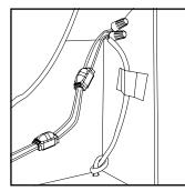
8. Connect power supply to first module on string: See power supply install guide for more information regarding power supply installation.
