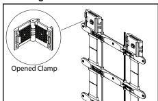
4a. Mounting modules with SignBOX II Clamps (P/N 410155) directly to cabinet: Insert straps from both sides of module into clamps (track features facing away from mounting surface) making sure clamps are flush against module, snap closed (avoid pinching wires), and secure to cabinet structure using #8 (M4) tek screws\*. Repeat on opposite end making sure product is taut.
