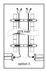
5. Using electrical connectors with appropriate safety agency markings, daisy chain product as required and connect to power supply as shown above. CAUTION! Have a licensed electrician connect primary. ATTENTION! Demandez à un électricien agréé de connecter le primaire. Modules may be connected in series or parallel. End wires of SignBOX II should be capped and not tied back to power supply.
