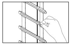
4c. Optional mounting in single-sided cabinet with double stick tape: Using non-oil based cleaner, clean all mounting surfaces of sign and bottom of modules for proper tape adhesion. With double stick tape on bottom of modules, mount to back of cabinet. Make sure product is taut. (Double stick tape is not included.)
