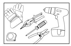
Tools required: Measuring tape, wire strippers, gloves, cutting tool (sheet metal shears/snips, scissors, utility knife), drill, and screwdriver.
