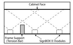
**NOTE:** To minimize the potential for shadows in applications when using frame support tubes, mount modules or frame support tubes such that the tubes are centered in between modules and at a depth that will not directly interfere with the beam angle of the LEDs.
