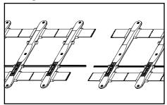
When cutting wires between modules, leaving one side longer will aid in joining product where needed. If, however, wires are not long enough for connections, use either jumper wires or remove a module to maximize wire length.
