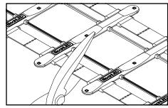
Cutting product: Cut straps (along dashed lines) and wires between modules to obtain required length. Tip: Before cutting wires, refer to Joining Product section.
