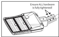
**3.** Tighten all mounting hardware and ensure luminaire is securely mounted.
