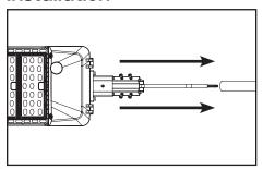
Loosen mounting hardware as necessary to position luminaire on 1.25" rigid conduit or 1.5" square tubing. Pull cable through mounting arm and pole for mounting.
