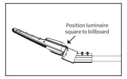
2. Ensure luminaire is fully seated against end of pole and ensure final position is square to surface to be illuminated.
