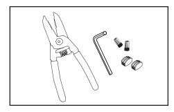
**Tools required:** UL Listed electrical connectors (wire nuts, lever nuts, etc.), 6 mm hex key, wire strippers.
